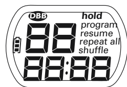
test pattern 2 (alternate segments activated)
