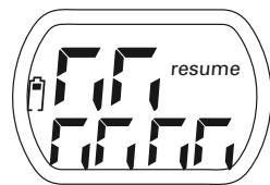
test pattern 2 (alternate segments activated)
